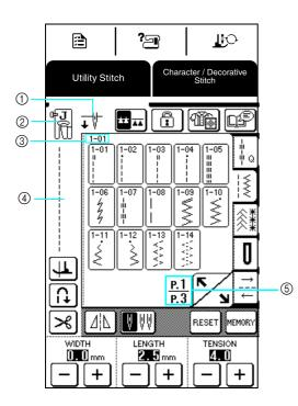
(1) Shows whether the machine is set for a single needle or twin needle, and the needle position when the machine is stopped. The desired needle position can be set (see page 22).
